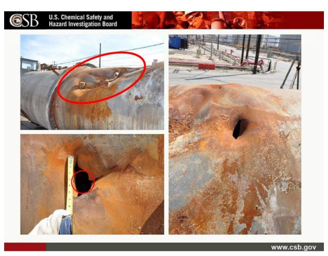
Figure 3 — Rupture of tank resulting from February 18, 2015 explosion at the Torrance refinery. The rupture shown in the lower-left image has the same flow area as a 3.65-inch-diameter hole, which has over 13 times the flow area of a 1-inch-diameter hole.
